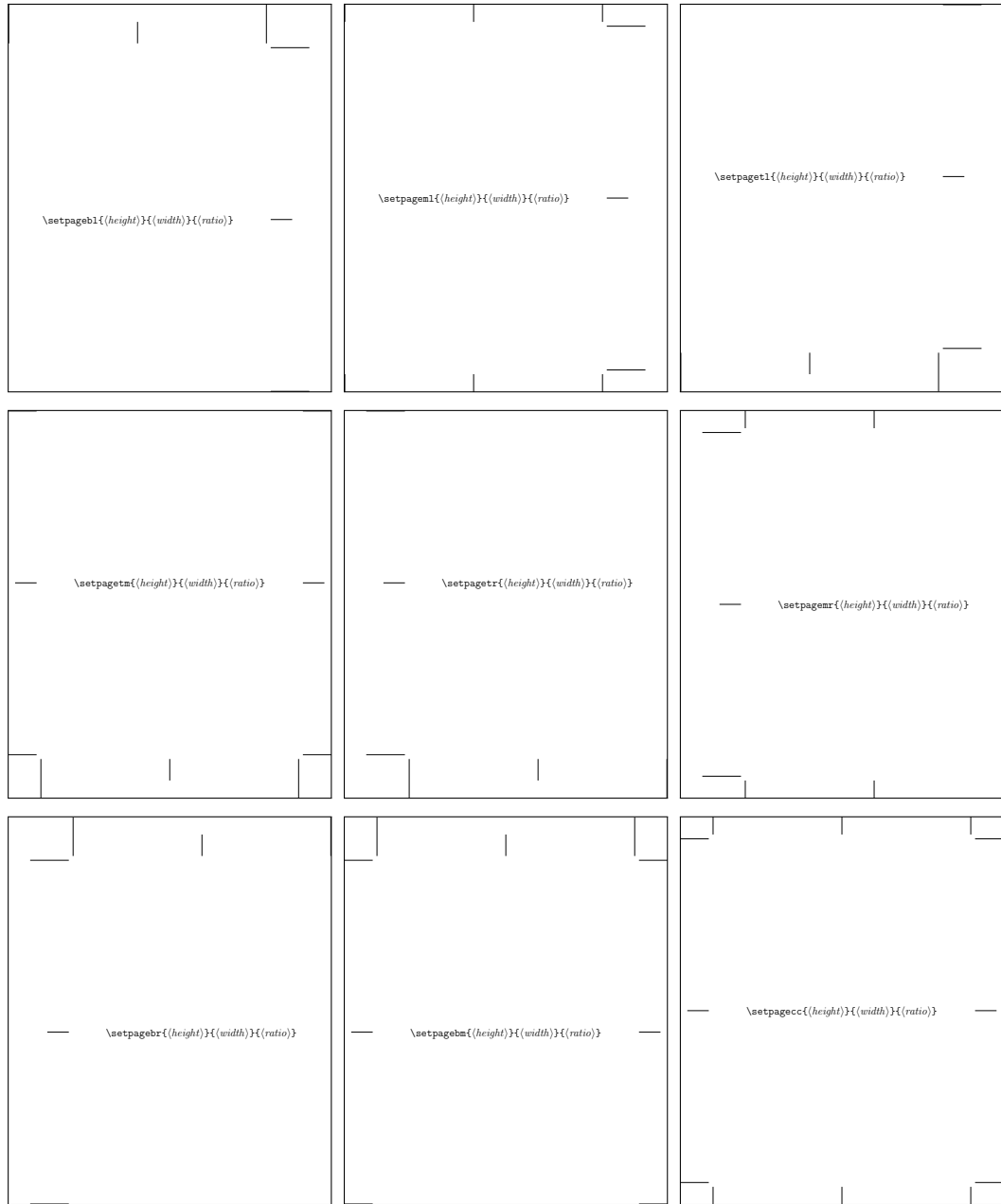
Figure 2.13: Example of the nine \setpageXX macros for placing a trimmed page on the stock. These are all odd pages, under twoside , even pages will have the left/right trims reversed. The outer frames indicate the stock size. Inside the trim marks hint at where the page is positioned on the stock.
